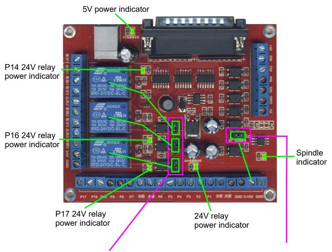
P14 Jumper, P16 Jumper, P17 Jumper. Remove these jumpers to disable the relays. Once disabled they can be used as a motor out pins.
