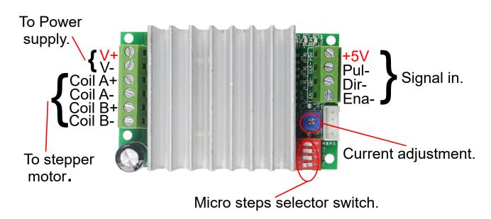
Note: If the input control voltage is 5V, then there is no current resistor needed. If the input control voltage is 12V, then use a 1.5K resistor for R\_EN, R\_CW, R\_CLK. If the input control voltage is 24V, then use a 3.0K resistor for R\_EN, R\_CW, R\_CLK
